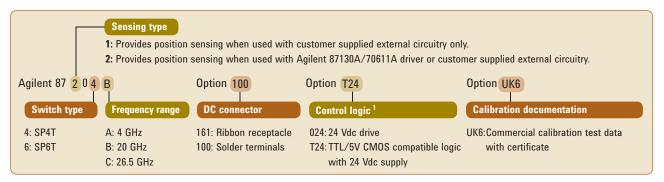
Here is an example of ordering system of Agilent switches. More detailed information can be found in the *Agilent Technologies RF and Microwave Test Accessory Catalog 2006-07*, literature number 5968-4314EN or in the technical overview for the switch model.
