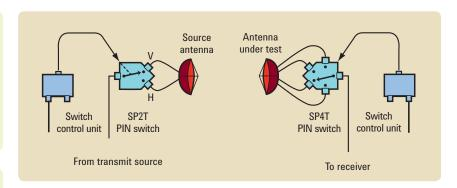
A typical multiple-channel, multiple-frequency system configuration
