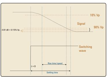
Switching waveform and settling time diagram
