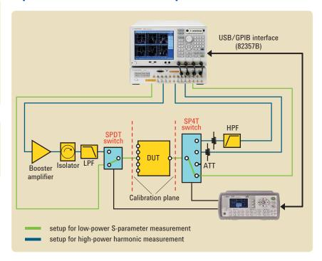
This configuration enables switching between high- and low-power measurements
