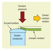
EM switch mating configuration illustrating microscopic wiping
