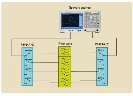
Typical test setup for filter bank testing
