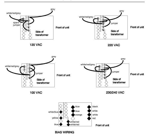
Figure 3-3. Transformer Wiring
