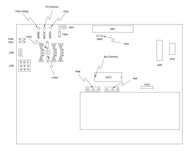
Figure 6-1. A1 Board Component and Test Point Locations
