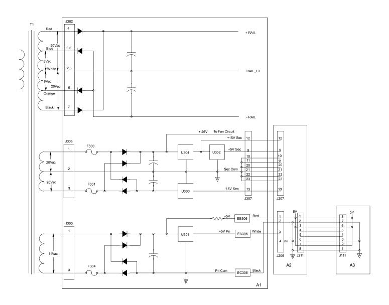
Figure 6-4. Rail and Bias Circuits
