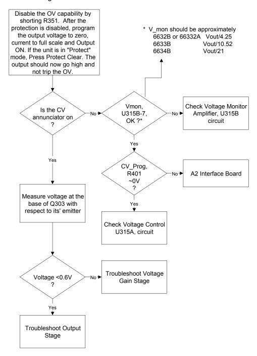
Figure 3-1 Sheet 12. High Output Voltage
