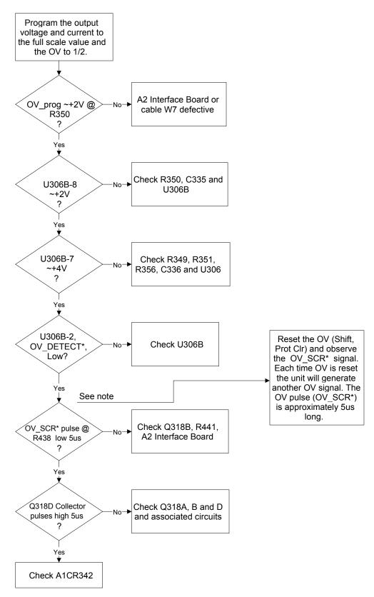
Figure 3-1 Sheet 11. Unit Does Not OV
