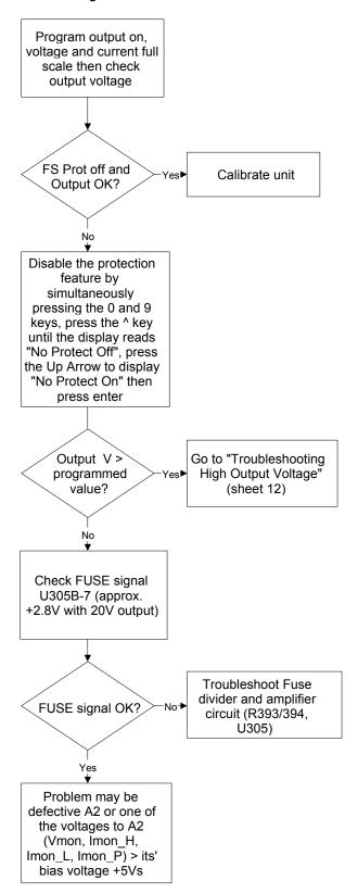
Figure 3-1 Sheet 6. FS Indicated but Fuse OK
