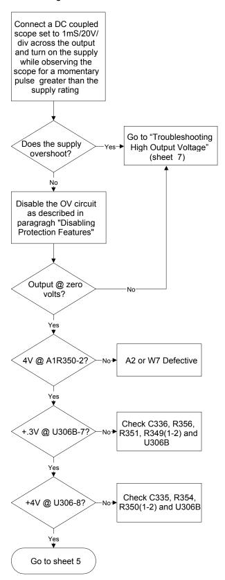
Figure 3-1 Sheet 4. OV at Turn-On
