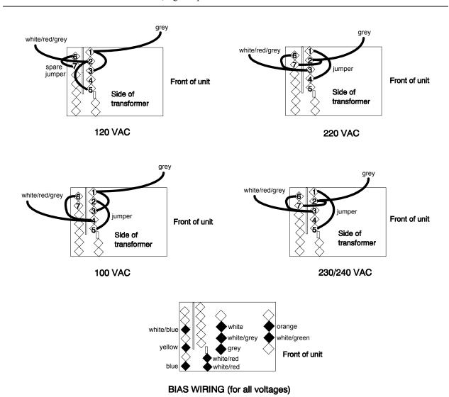
Figure 3-3. Transformer Wiring
