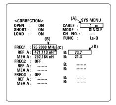
Figure 3. Correction function setup
