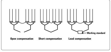
Figure 4. Performing correction measurements
