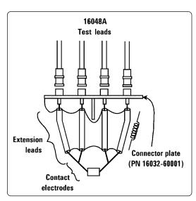
Figure 2 . Contact electrodes
