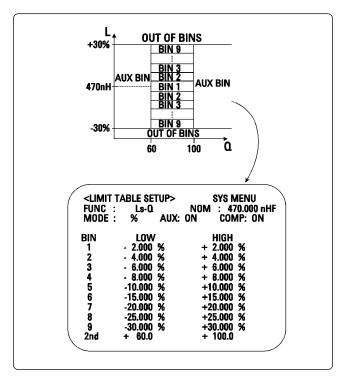
Figure 5 : Comparator setup
