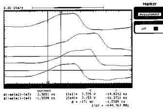
Figure 4. Skew in Clock Signal
