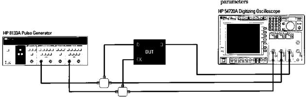
Test Setup for Characterizing a D Flip-Flop
