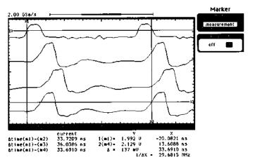
Figure 3. Path Delay in Clock Signal
