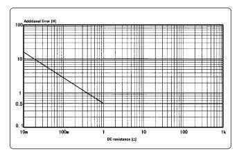
Figure 11. Dc resistance additional error
