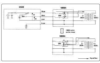
Figure 1. Agilent 4263B block diagram for L, M, and DCR measurement
