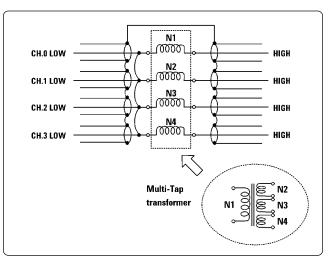
Figure 9. Connection of multi-tap transformer
