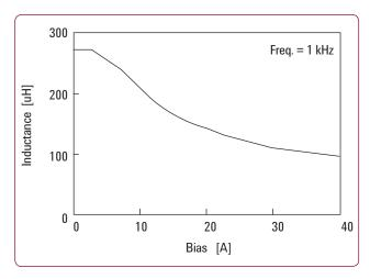
Figure 7. Measurement results up to 40  $\mbox{\ensuremath{\mbox{A}}}$
