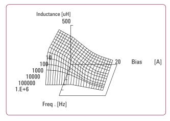
Figure 6. Frequency characteristics of L-IDC
