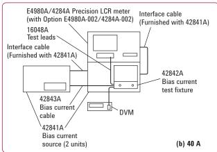
Figure 4. Measurement configuration
