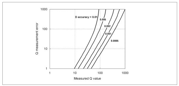
Figure 5-15. Q measurement accuracy
