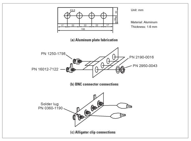
Figure 3-10. Example of fixture fabrication
