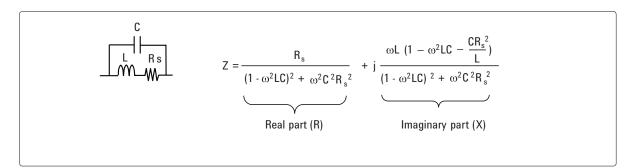
Figure 5-10. Inductor equivalent circuit
