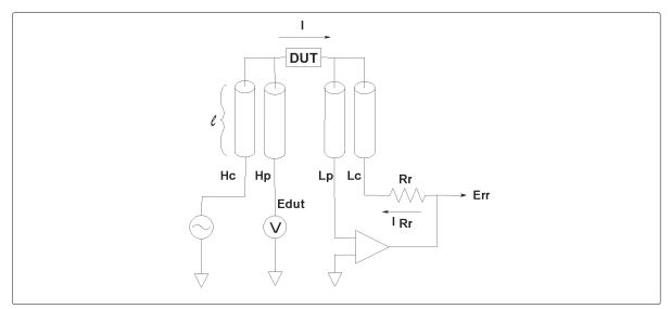
Figure 4-11. Cable length correction
