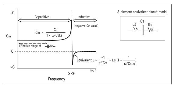
Figure 1-18. Influence of parasitic inductance on capacitor
