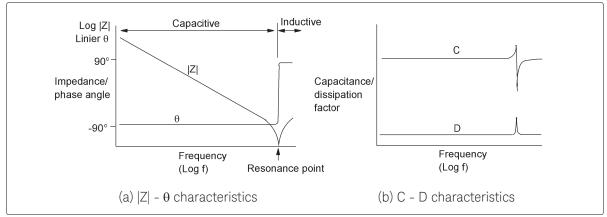
Figure 5-5. Typical capacitor frequency response
