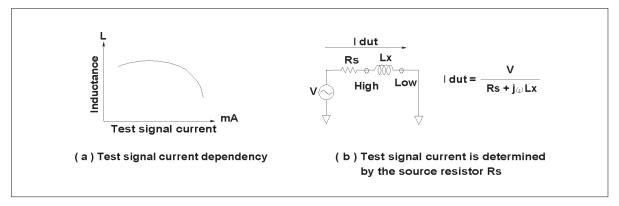
Figure 5-13. Inductor test signal current
