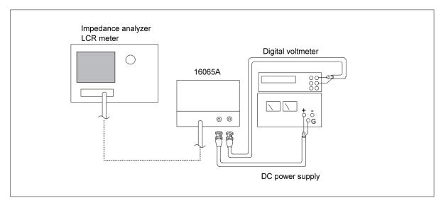
Figure 5-45. External DC bias measurement setup
