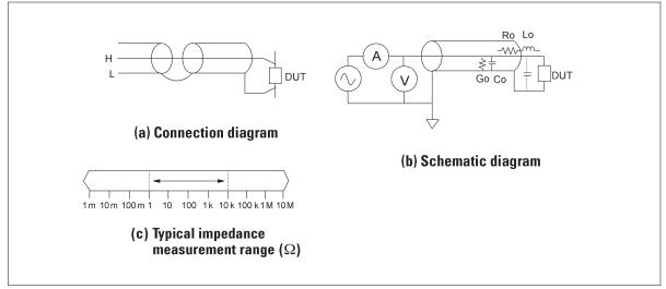
Figure 3-17. Coaxial test port circuit configuration
