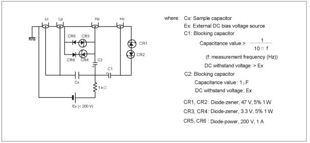
Figure 5-46. External DC voltage bias protection circuit
