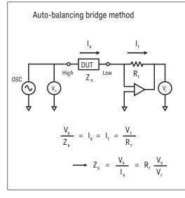
The current Ix balances with the current Ir which flows through the range resistor (Rr), by operation of the I-V converter. The potential at the Low point is maintained at zero volts (thus called a virtual ground.) The impedance of the DUT is calculated using the voltage measured at the High terminal (Vx) and across  $R_r$  (Vr).
