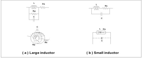
Figure 5-9. Inductor equivalent circuit
