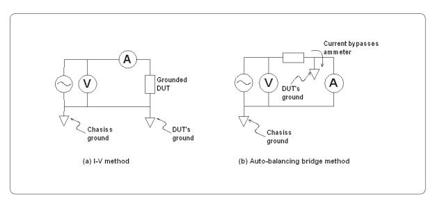
Figure 2-12. Low-grounded device measurement
