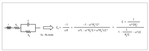
Figure 5-3. Effects of parasitics in actual capacitance measurement
