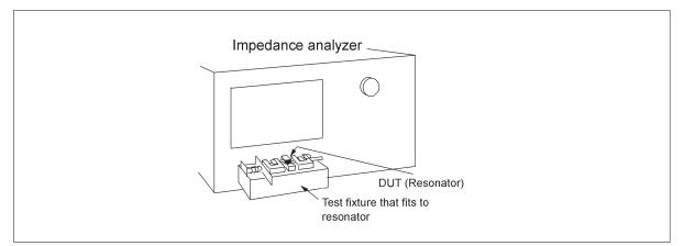
Figure 5-35. Resonator measurement setup
