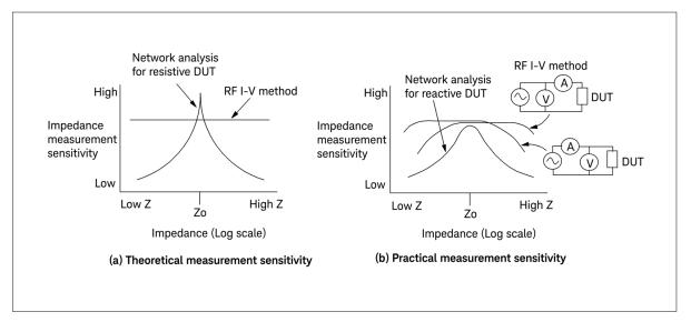
Figure 2-15. Measurement sensitivity of network analysis and RF I-V methods
