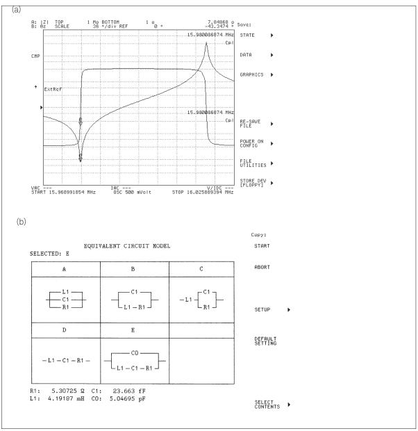
Figure 5-36. Resonator equivalent circuit mode on 4294A
