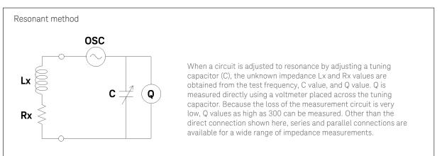
Figure 2-1. Impedance measurement method (1 of 3)
