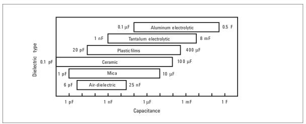
Figure 5-1. Capacitance value by dielectric type
