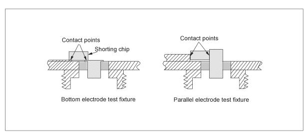
Figure 4-20. Difference in short impedance by test fixture types
