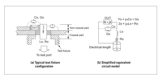
Figure 4-15. Typical error source model
