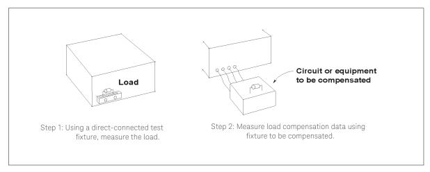
Figure 4-9. Actual open/short load measurement example
