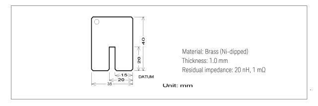
Figure 4-5. Example of shorting device (Keysight part number 5000-4226)
