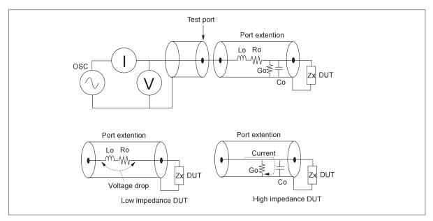
Figure 3-19. Calibration plane extension
