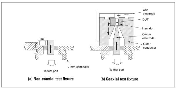
Figure 3-18. Types of RF impedance test fixtures
