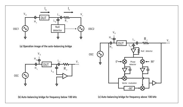
Figure 2-4. Auto-balancing bridge section block diagram
