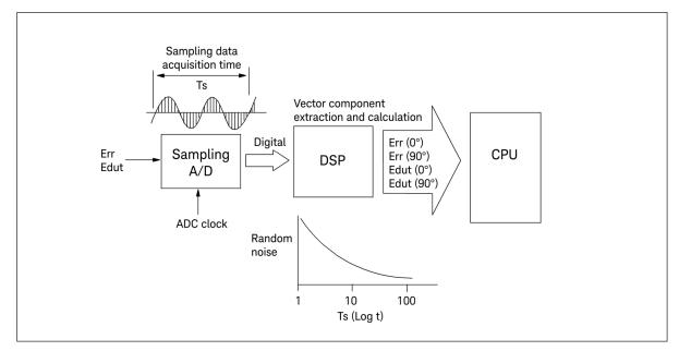
Figure 2-10. Relationship of measurement time and precision
