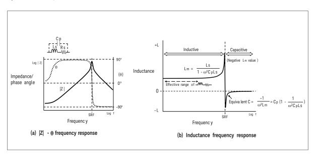
Figure 5-12. Typical inductor frequency response
