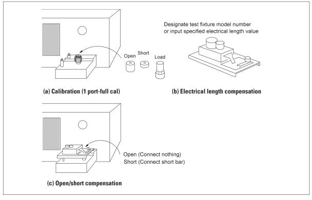
Figure 4-17. Complete calibration and compensation procedure
