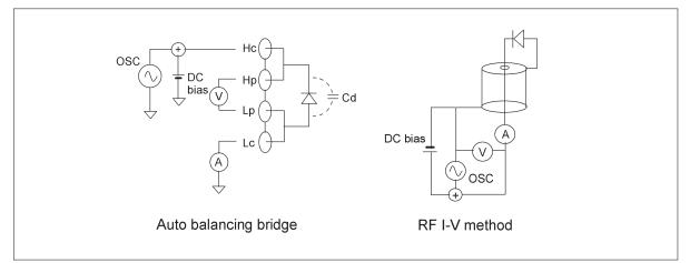
Figure 5-26. Reverse biased diode measurement setup
