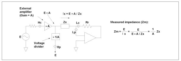
Figure 5-43. Schematic diagram of test signal voltage enhancement circuit
