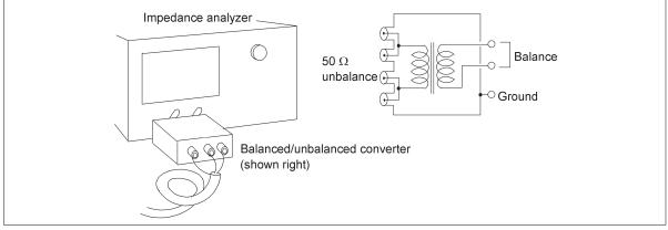
Figure 5-39. Balanced cable measurement setup
