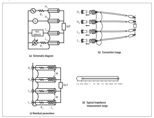
Figure 3-6. Five-terminal (5T) configuration
