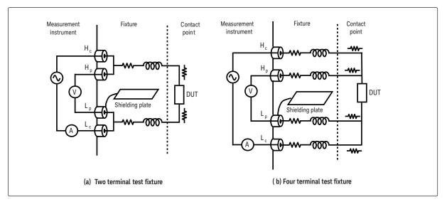
Figure A-5. Two-terminal and four-terminal connection techniques
