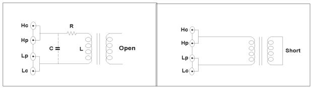
Figure 5-19. Primary inductance measurement
