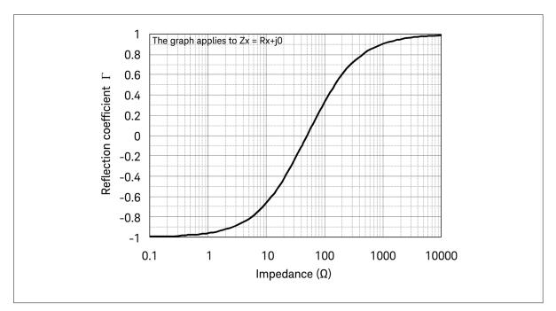
Figure 2-14. Relationship of reflection coefficient to impedance
