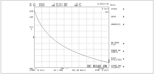
Figure 5-27. Varactor C-V characteristics
