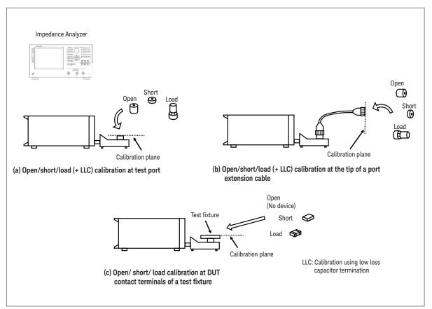
Figure 4-2. Calibration plane of RF-IV instruments
