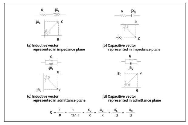
Figure 1-4. Relationships between impedance and admittance parameters
