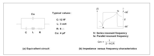
Figure 5-34. Typical resonator characteristics
