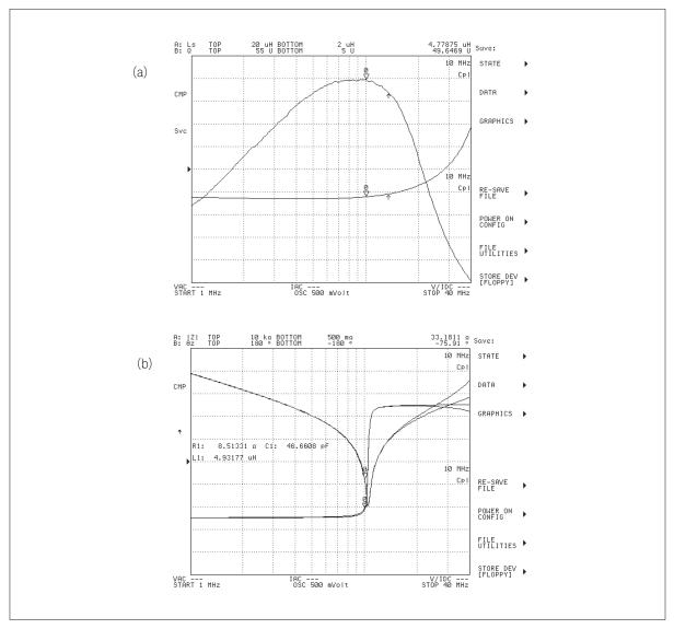
Figure 5-52. Q measurement accuracy improvement
