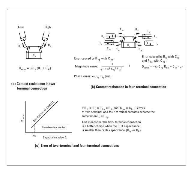
Figure 4-10. Effect of contact resistance
