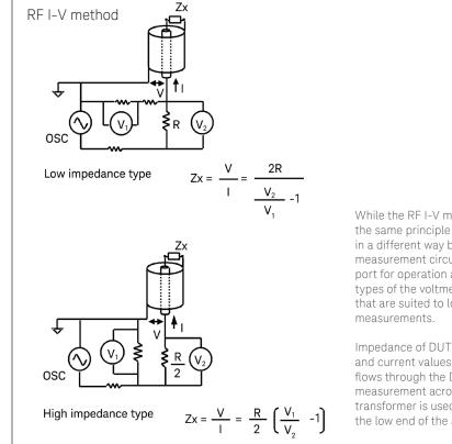
While the RF I-V measurement method is based on the same principle as the I-V method, it is configured in a different way by using an impedance-matched measurement circuit (50  $\Omega$ ) and a precision coaxial test port for operation at higher frequencies. There are two types of the voltmeter and current meter arrangements that are suited to low impedance and high impedance measurements.
