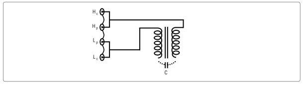
Figure 5-21. Inter-winding capacitance measurement
