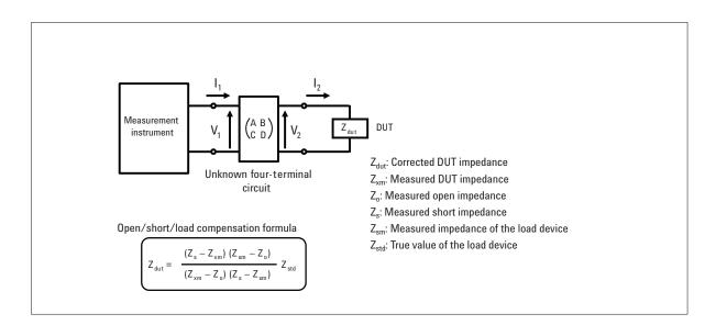
Figure 4-6. Open/short/load compensation
