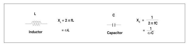
Figure 1-3. Reactance in two forms: inductive  $(X_1)$  and capacitive  $(X_2)$
