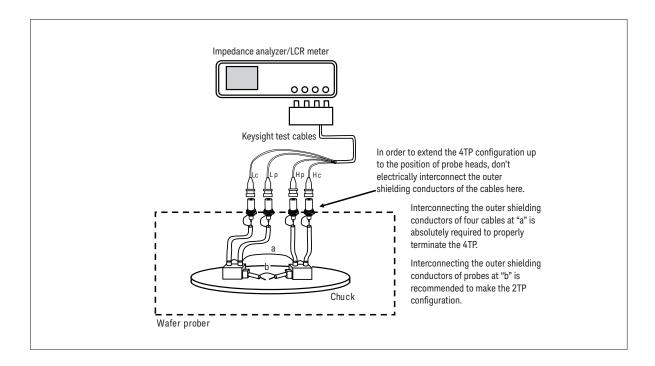
Figure 5-30. C-V measurement setup using 4TP cable extension
