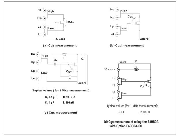
Figure 5-29. MOS capacitance measurement
