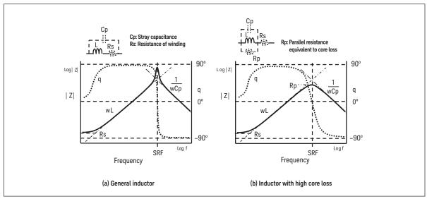
Figure 1-8. Inductor frequency response
