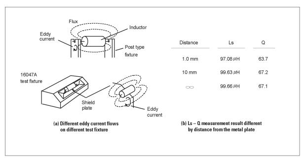
Figure 5-14. Test fixture effects
