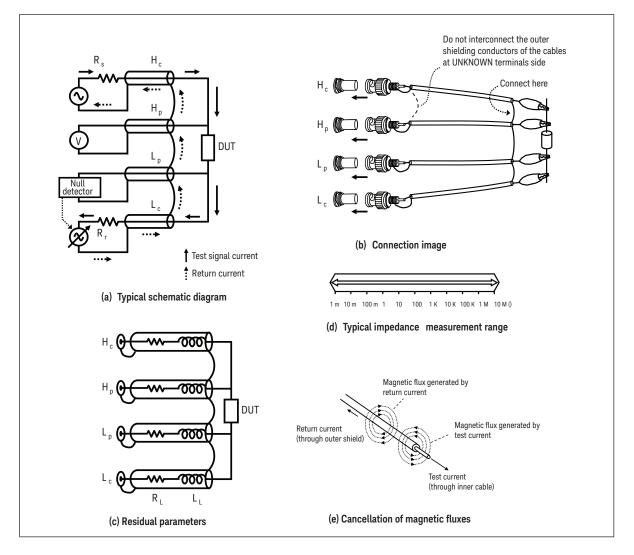
Figure 3-8. Four-terminal pair (4TP) configuration
