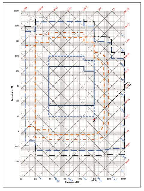
Figure 1-21. Example of measurement accuracy indicated on a reactance chart
