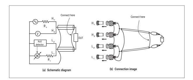
Figure 3-4. Shielded two-terminal (2T) configuration
