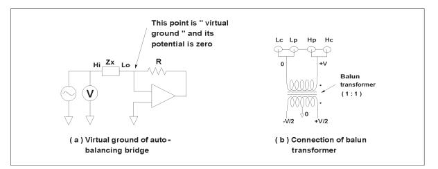
Figure 5-40. Balanced device measurement
