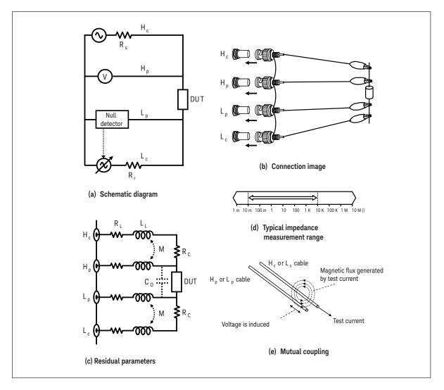
Figure 3-5. Four-terminal (4T) configuration
