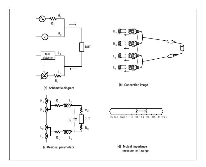
Figure 3-2. Two-terminal (2T) configuration
