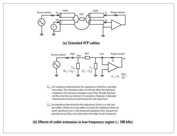
Figure 4-12. Measurement error due to extended cable length
