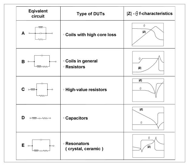
Figure 5-49. Equivalent circuit models on 4294A
