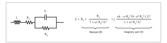
Figure 5-2. Capacitor equivalent circuit
