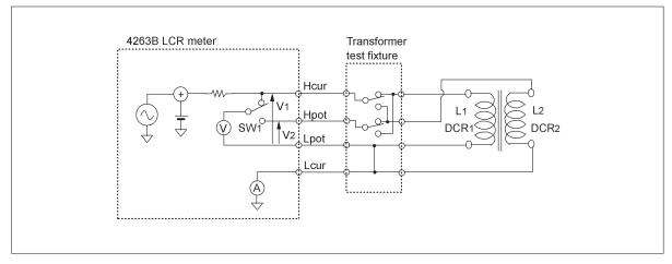
Figure 5-25. 16060A circuit connection diagram
