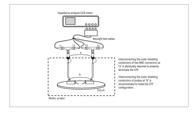
Figure 5-31. C-V measurement setup using 2TP cable extension
