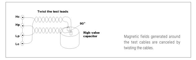
Figure 5-6. High-value capacitor measurement
