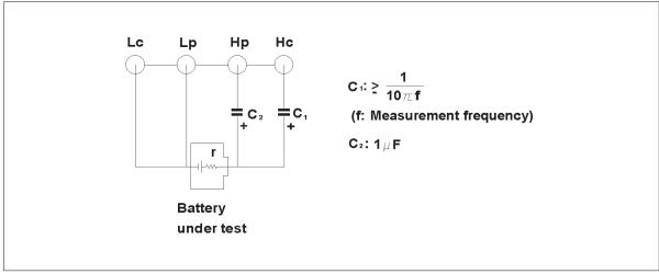
Figure 5-42. Battery measurement setup
