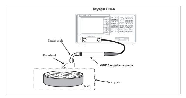
Figure 5-32. Example of high-frequency C-V measurement system configuration
