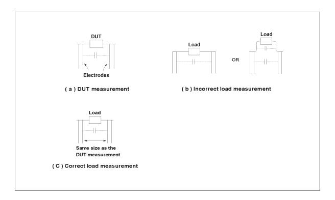
Figure 4-7. Electrode distance in load measurement
