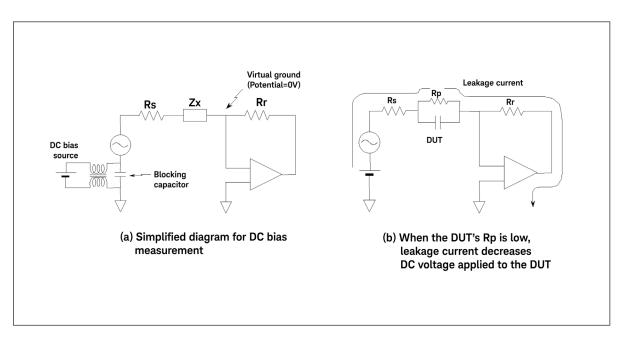
Figure 2-7. DC bias applied to DUT referenced to virtual ground
