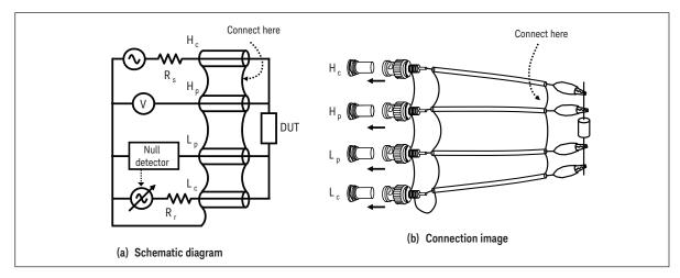
Figure 3-7. Shielded four-terminal (4T) configuration
