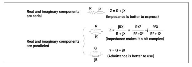
Figure 1-2. Expression of series and parallel combination of real and imaginary components
