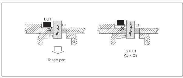
Figure 4-18. Difference in residual parameter values due to DUT positioning
