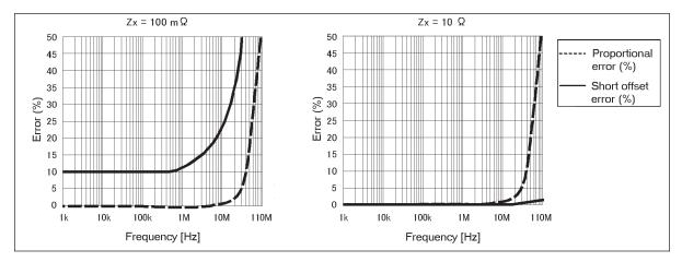
Figure A-4. Relationship between proportional error, short offset error, and frequency when measuring low impedance
