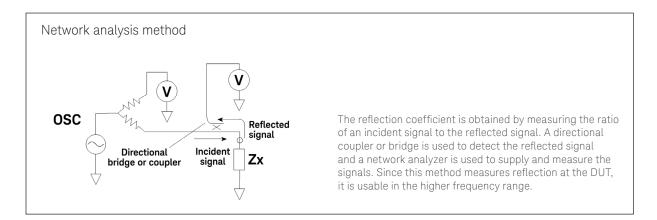
Figure 2-1. Impedance measurement method (2 of 3)
