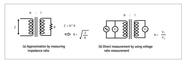
Figure 5-23. Turns ratio measurement
