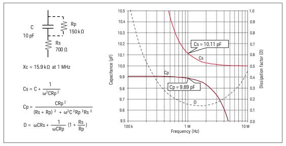
Figure 1-19. Example of capacitive device affected by both Rs and Rp
