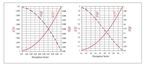
Figure 1-16. Relationships of series and parallel capacitance values
