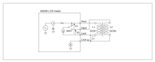
Figure 5-24. 4263B transformer measurement function schematic block diagram
