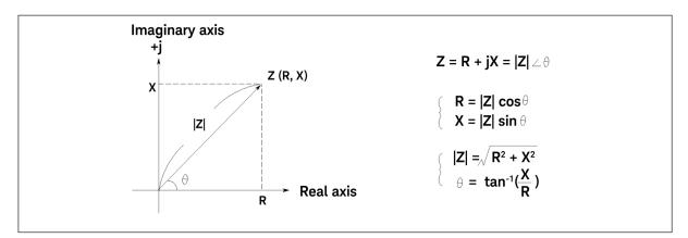
Figure 1-1. Impedance (Z) consists of a real part (R) and an imaginary part (X)
