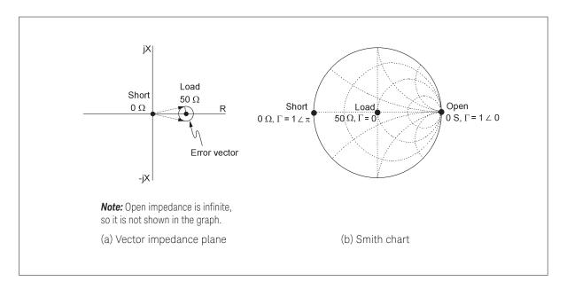
Figure 4-14. Calibration standard values
