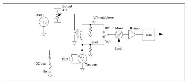
Figure 2-13. Simplified block diagram for RF I-V method
