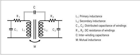
Figure 5-18. Transformer parameters
