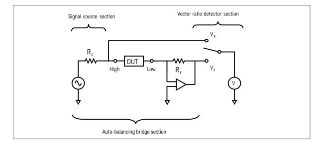
Figure 2-3. Impedance measurement using a single vector voltmeter
