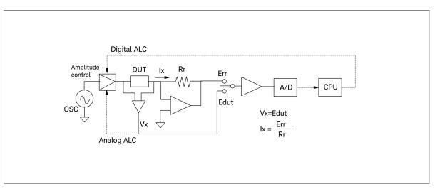
Figure 2-9. Test signal level monitor and ALC function
