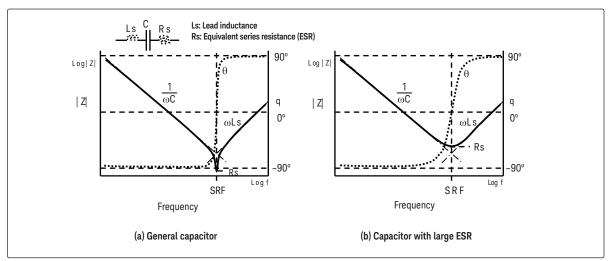
Figure 1-7. Capacitor frequency response
