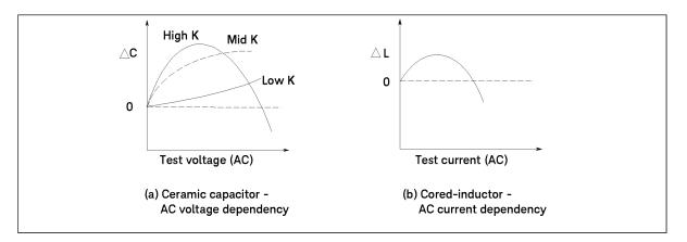
Figure 1-10. Test signal level (AC) dependencies of ceramic capacitors and cored-inductors
