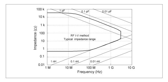
Figure 4-16. Relationship of residual parameter values to the typical impedance measurement range of the RF I-V method
