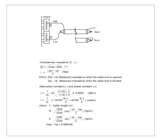
Figure 5-37. Coaxial cable measurement setup and parameter calculation
