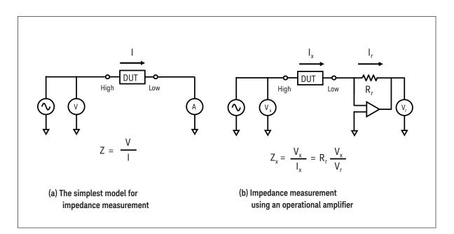
Figure 2-2. Principle of auto-balancing bridge method
