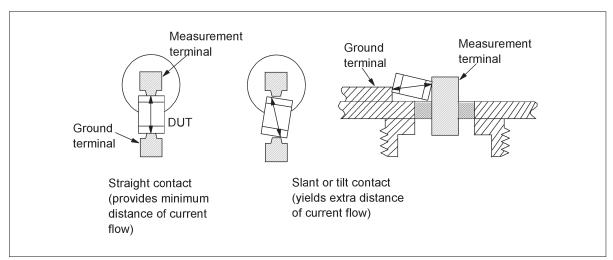
Figure 4-19. Measurement error caused by improper DUT positioning
