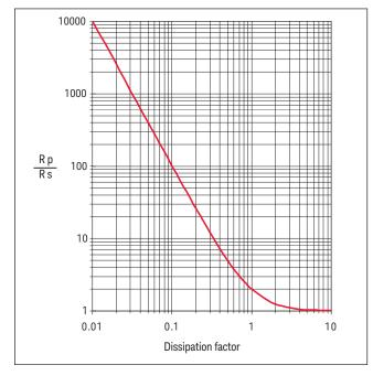
Figure 1-17. Relationships of series and parallel resistance values
