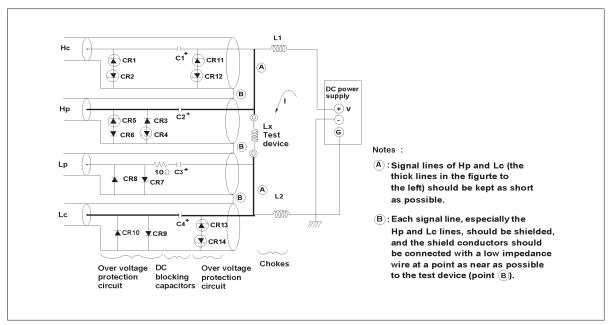
Figure 5-48. External current bias protection circuit
