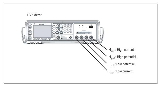
Figure 3-1. Measurement terminals of auto balancing bridge instrument
