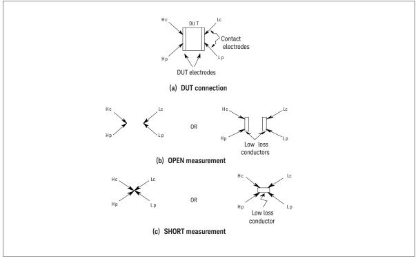
Figure 3-9. User-fabricated test fixture open/short methods
