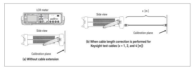
Figure 4-1. Calibration plane of auto-balancing bridge instruments
