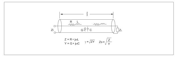
Figure D-1. Transmission line model of test port extension
