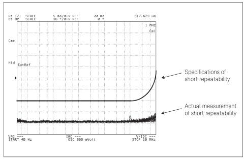
Figure A-6. Measurement of short repeatability (16034G)
