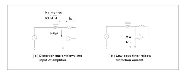
Figure 5-17. Harmonic distortion caused by inductors
