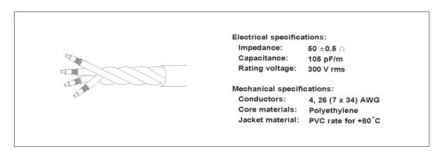
Figure 3-11. Specifications of recommended cable (Keysight part number 8121-1218)
