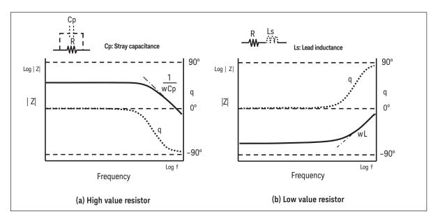
Figure 1-9. Resistor frequency response
