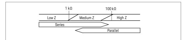
Figure 1-15. High and low impedance criteria
