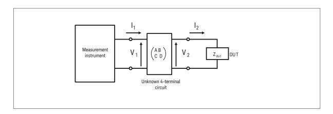
Figure B-1. Four-terminal network circuit model of a test fixture or test cables
