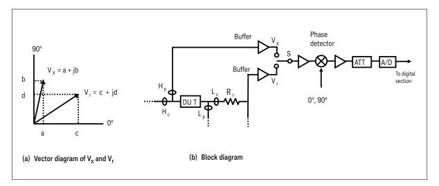
Figure 2-5. Vector ratio detector section block diagram
