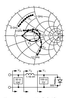
Figure 13. Detector Matched with Shunt Transmission Line, 50  $\mu A$  Bias, Admittance Coordinates.
