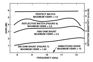
Figure 8. Gain of Detector Matching Networks.
