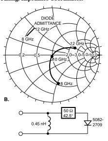
Figure 2B. Single Frequency Shunt Tuning, Admittance Coordinates.
