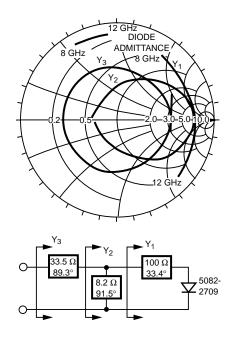
Figure 6. Matching the Detector Diode, 50  $\mu$ A Bias, Admittance Coordinates.
