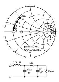
Figure 1. Admittance of 5082-2709 Beam Lead Mixer. 1.5 mA Rectified Current.
