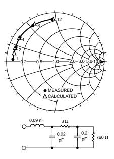
Figure 5. 5082-2709 Beam Lead Diode Admittance, 50  $\mu A$  Bias.
