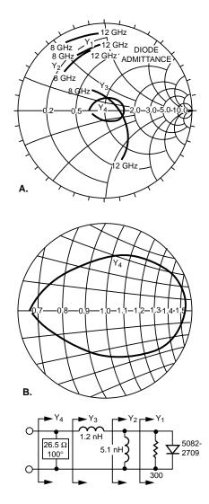
Figure 11. Detector Matching with Shunt Inductance, 50  $\mu$ A Bias, Admittance Coordinates.
