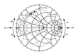
Figure 10. Detector Matching on Immittance Chart.
