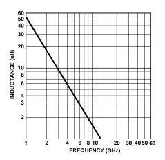
Figure 12. Maximum Inductance of Microstrip Coils.
