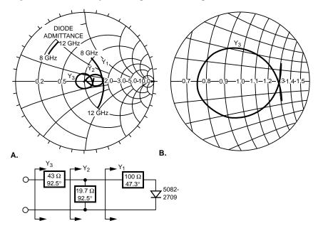
Figure 4. Three Element Mixer Matching Circuit, Admittance Coordinates.
