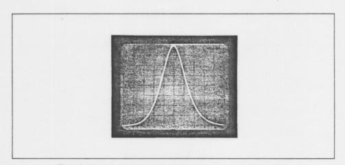
Figure 5. Display adjusted so that the filter response almost fills the CRT.
