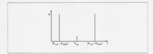
Figure 22. Output of the mixer when local oscillator and test oscillator are unlocked.
