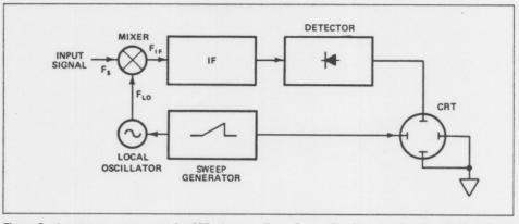
Figure 2. A response appears on the CRT whenever F,  $\pm$   $F_{1\circ}$  =  $F_{1F}$ . Example: For the 8553B 110 MHz Spectrum Analyzer,  $F_{1F}$  = 200 MHz;  $F_{*}$  = 0 - 110 MHz; and  $F_{L\circ}$  = 200 - 310 MHz. Then, for an input signal at 50 MHz, the local oscillator would be tuned to 250 MHz to get a 200 MHz difference frequency and a response on the CRT.
