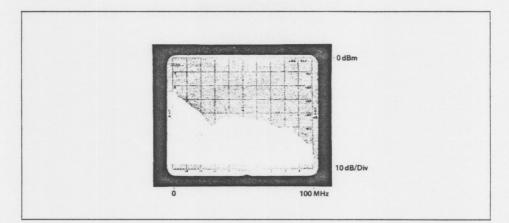
Figure 6. Example: Impulse noise level at 70 MHz is -47 dBm. We add 107 dB to get +60 dB $\mu$ V. Subtracting the bandwidth correction factor, we get 77.1 dB $_{\mu}$ V/MHz.
