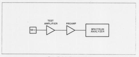
Figure 15. Noise figure test setup.
