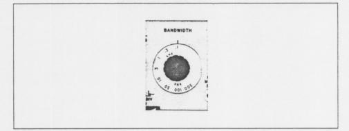
Figure 9. The setting of the bandwidth control is the nominal 3 dB bandwidth of the spectrum analyzer.
