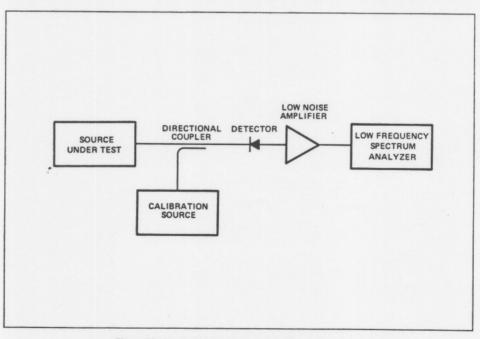
Figure 19. Block diagram for residual AM measurements.
