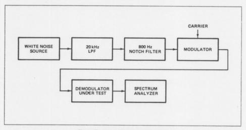
Figure 17. Basic white noise loading test.
