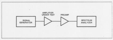
Figure 14. Test setup to calibrate the gain of the two amplifiers.
