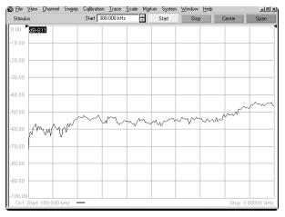
Figure 11. Measurement of load standard after calibration
