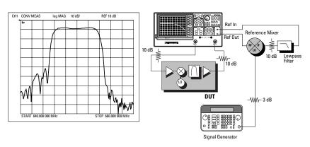
Figure 7B. High dynamic range conversion loss measurement (left) and high dynamic range setup (right)
