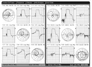
Figure 14. Single-ended and corresponding mixed-mode measurement parameters
