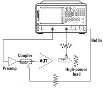
Figure 2. High-powered foward measurement configuration
