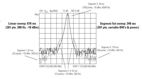
Figure 12. Optimize filter measurements with segment list mode
