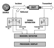
Figure 1. Network analyzer block diagram
