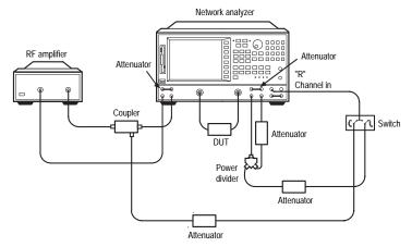
Figure 3. High-powered forward and reverse measurement configuration
