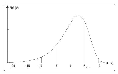
Figure 6. The PDF of logged noise is about 30 dB wide and tilted toward the high end.
