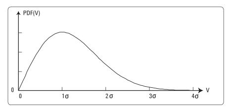
Figure 4. The PDF of the voltage of the envelope of a noise signal is a Rayleigh distribution. The PDF is zero at zero volts, even though the PDFs of the individual I and  $\Omega$  components are maximum at zero volts. It is maximum for v = sigma.
