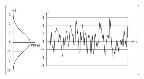
Figure 1. The Gaussian PDF is maximum at zero current and falls off away from zero, as shown (rotated 90 degrees) on the left. A typical noise waveform is shown on the right.
