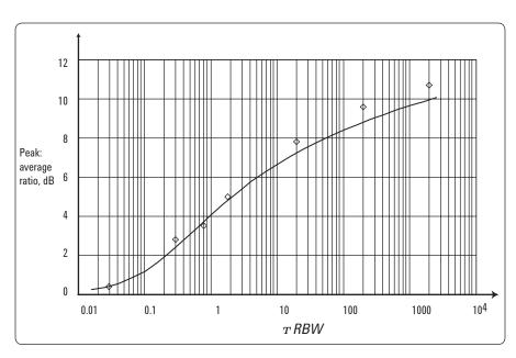
Figure 14. The peak-detected response to noise increases with the observation time.
