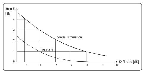
Figure 20. CW signals measured on a logarithmic scale show very little effect due to the addition of noise signals.
