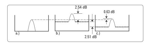
Figure 18. Log averaging improves the measurement of CW signals when their amplitude is near that of the noise. (a) shows a noise-free signal. (b) shows an averaged trace with power-scale averaging and noise power 1 dB below signal power; the noise-induced error is 2.5 dB. (c) shows the effect with log-scale averaging—the noise falls 2.5 dB and the noise-induced error falls to only 0.6 dB.
