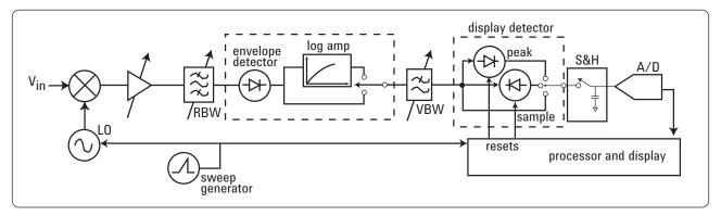
Figure 8. Simplified spectrum analyzer block diagram
