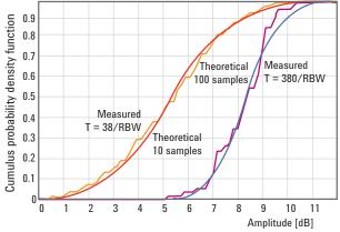
Figure 16. Setting N a factor of 3.8 below the product of the observation time and the RBW gives good agreement between experiments with continuous time systems and theory for independent samples in this CDF plot.
