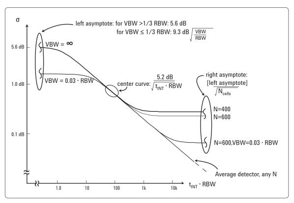
Figure 17. Noise measurement standard deviation for log-response (see text for power-response) spectrum analysis depends on the product of the sweep time and RBW, the ratio of the VBW to RBW, and the number of display cells.
