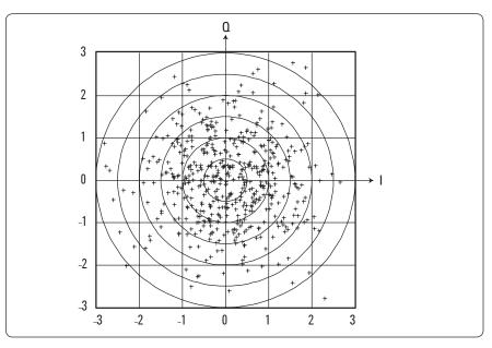
Figure 3. Samples of I/O pairs shown with evenly spaced constant-amplitude envelope circles
