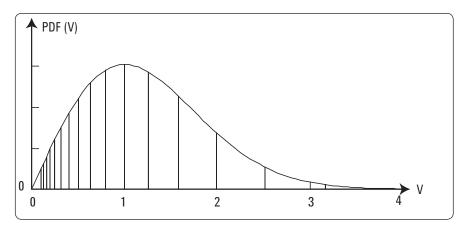
Figure 5. The PDF of the voltage envelope of noise is graphed. 1 dB spaced marks on the x-axis shows how the probability density would be different on a log scale. Where the decibel markings are dense, the probability that the noise will fall between adjacent marks is reduced.
