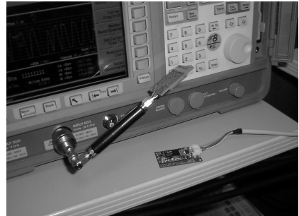
Figure 16. Picture of Agilent ESA-E spectrum analyzer receiving a Bluetooth signal over the air using a RangeStar Bluetooth antenna
