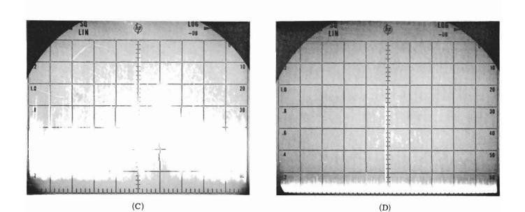
Figure 1. (A) Shows an abrupt recovery diode harmonic generator setup. Parametric Oscillations and noise outputs shown in (B) and (C). Picture (D) shows proper 3800 mc output. Vertical 10 db/cm allows good readability of undesired signals.
