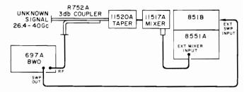
Figure 19. Setup for more sensitivity in 26 - 40 gc range.
