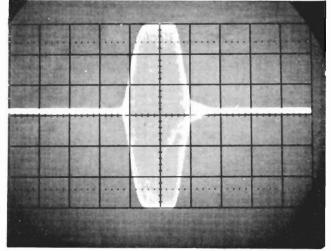
(D) The RF pulse has a voltage pulse width of slightly over 3  $\mu sec$  agreeing with the analyzer prediction.
