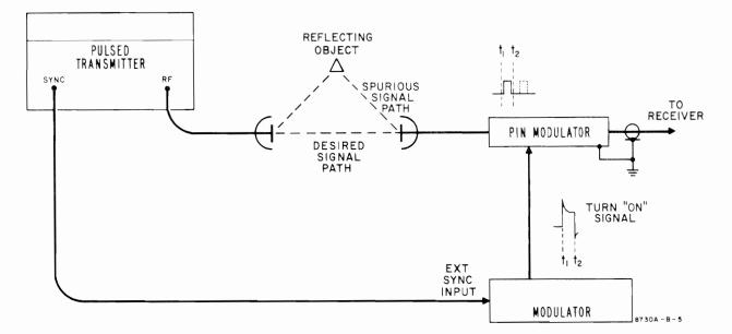
Figure 17. Multiple antenna interference may be minimized by a synchronizing gate.
