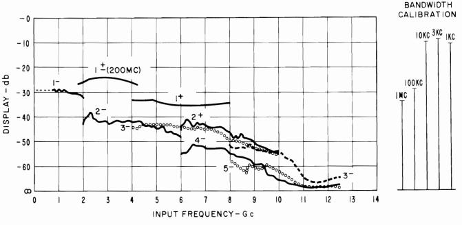
Figure 14. Sensitivity calibration for various harmonic mixing modes.
