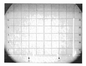
Figure 4. The 1800 mc generator output is on the right in the n = 1<sup>-</sup> band. 3600 mc harmonic left of center is in the n = 2<sup>-</sup> band. Horizontal 200 mc/cm, vertical 10 db/cm.
