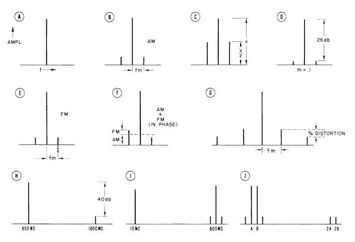
Figure 11. Typical modulation and distortion spectra. See Text.
