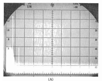
Figure 3. Picture (A) shows normal 150 mc transistor amplifier output. (B) shows amplifier overloaded with distortion products. Horizontal 200 mc/cm, vertical 10 db/cm.
