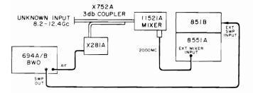
Figure 18. -hp- 694 series sweeper can be used to get fundamental mixing from 8 - 12.4 gc.
