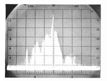
This is a display of a 1 megawatt radar at mid-L band showing spurious radiation over 300 mc below the main carrier and interfering in TACAN channels. Horizontal 100 mc/cm, vertical 10 db/cm. Some emitted broadband output is only 20 db down from carrier (10 kw).
