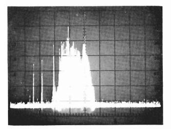
Magnetron output; 100 mc/cm
