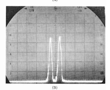
Figure 10. These photos show the increased resolution possible with the -hp- 8442A 1 kc filter. (A) Normal 1 kc BW. (B) 8442A installed. Horizontal scale 10 kc/cm, at 150 mc, vertical 10 db/cm.
