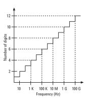
Figure 2. The number of digits displayed by a direct counter versus frequency (for a 1 second gate time).
