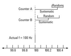
Figure 1. Simplified view of resolution vs. accuracy. Systematic errors related to the timebase "push" the displayed frequency away from the actual frequency. The random errors create a range of frequencies inside of which the counter can't distinguish different signals.
