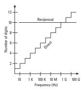
Figure 4. Here are the gate times needed to yield various resolutions with a 10 digits/second reciprocal counter.
