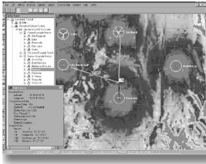
The WIZARD software is a versatile, full-featured wireless network planning tool. It is shown here in multiple servers analysis mode, displaying four strongest servers.
