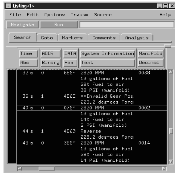
A custom tool extracts system information from the ADDR and DATA trace and converts it to easily understood text that speeds insight into system problems.
