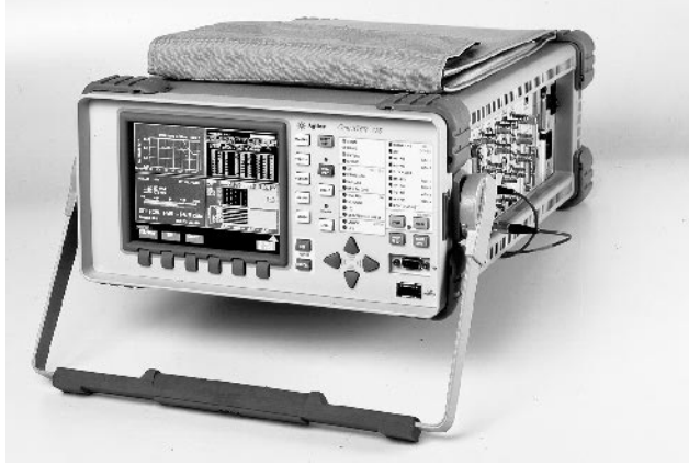
New, portable OmniBER 725 provides optical and differential electrical interfaces for testing fiber optic transmitter (E/O) and receiver (O/E) modules.
