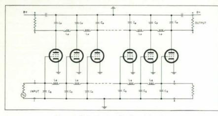
Figure 2. Basic Circuit of Distributed Amplifier
