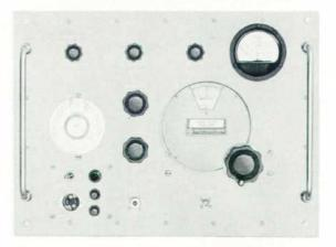
Figure 1. Panel view of -bp- Model 618A 3800-7600 Mc Signal Generator.
