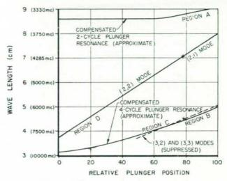
Figure 5. Frequency plot of uncompensated parallel-plane oscillator.
