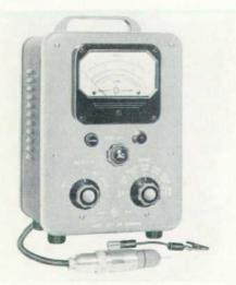
Figure 1. New -bp- Model 410B High-Frequency VTVM supersedes widely-used Model 410A. In addition to electrical improvements, the instrument has been completely redesigned mechanically. Leads are stored in compartment at back of cabinet.
