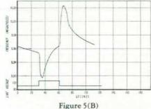
change in frequency when line voltage is changed and is further investigated in Figure 5(b) where measurements are made at 2-second intervals to magnify discontinuous area. Such measurements are typical of those that can be made with Model 524A.
