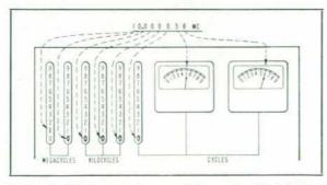
Figure 1. Display arrangement of new -bp- Model 524A Frequency Counter. Columns of neon tubes behind panel slots illuminate the proper numerals which are reverseprinted on transparent plastic. Example shown represents a frequency of 10,000,056 cps counted for period of one second. Maximum rate for instrument is 10 mc; maximum counting period is 10 seconds.
