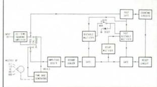
Figure 8. Block diagram of -hp- Model 524A Frequency Counter.
