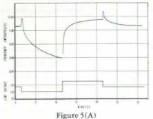
Frequency shift in -hp- Model 650A Test Oscillator operating at 10 mc when subjected to  $\pm$ 15-volt line change. Measurements made at 20-second intervals. Discontinuous curve results from sudden
