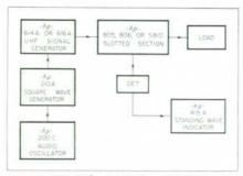
Fig. 3. Typical set-up for standing-wave measurements using -bp- Model 614A or 616A. Use of bigh-gain Model 415A Standard Wave Indicator increases sensitivity of measurements.
