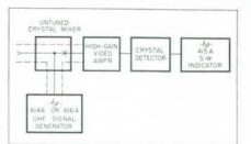
Fig. 4. Simple laboratory receiver using -bp- Model 614A or 616A as local oscillator.
