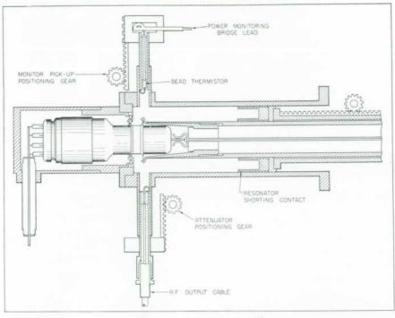
Fig. 6. Cross-section of UHF oscillator.
