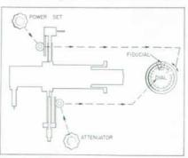
Fig. 7. Schematic representation of mechanical system for selecting and indicating output power level.
