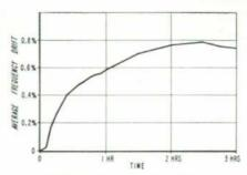
Fig. 4. Typical warm-up drift of new -bp- Model 200AB.
