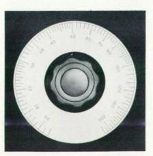
Fig. 8. Frequency dial of -bp- Model 200AB.
