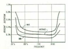
Fig. 3. Distortion measured on 20 production 200AB's. Curves show maximum and minimum values measured and average of all measurements.
