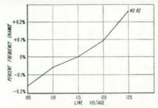
Fig. 6. Over most of frequency range line voltage effects are negligible. Above curve shows line voltage effect at highest operating frequency of 200AB where effect is most pronounced.
