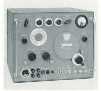
Fig. 1. New -bp- Model 620A SHF Signal Generator provides for cw, pulse, square-wave or f-m output over 7 to 11 kmc range.
