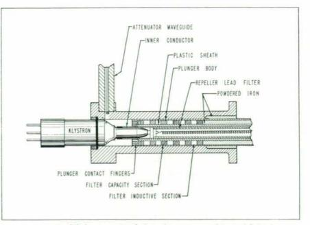
Fig. 3. Simplified cross-sectional view of resonator used in Model 620A.
