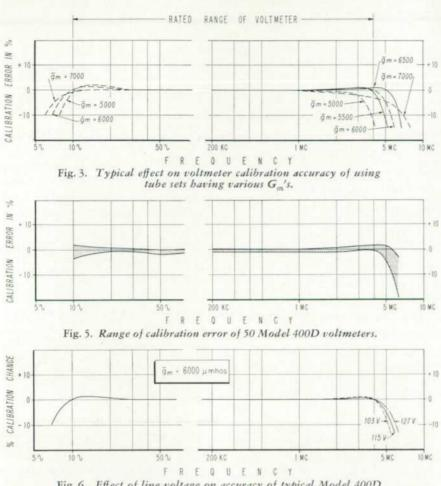
Fig. 6. Effect of line voltage on accuracy of typical Model 400D.
