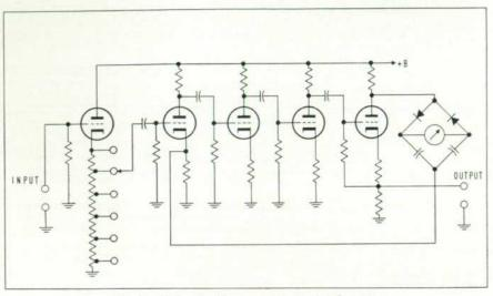
Fig. 2. Basic circuit arrangement of voltmeter.
