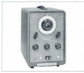
Fig. 1. New -bp- Model 211A Square Wave Generator operates from 1 cps to 1 megacycle, bas only 20 millimicroseconds rise time from fast output. A second output provides up to 55 volts peak-to-peak.
