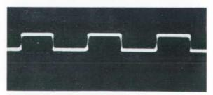
Fig. 2. Oscillogram of fast output from -hp-211A when operating at repetition rate of 1 megacycle into a 75-ohm resistive load.
