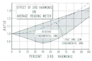
Fig. 5. Calculated limits of absolute average values of wave consisting of fundamental with various amounts of third harmonic. Small circles show experimental verification of calculated data.
