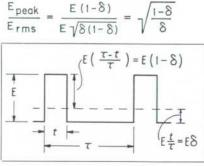
Fig. 8. Pulse waveform defining values used in text.
