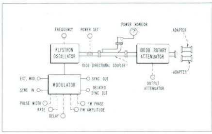
Fig. 2. Basic circuit arrangement of -bp- 628A Signal Generator.
