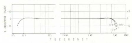
Fig. 3. Effect on voltmeter reading of  $\pm 10\%$  line voltage variation.
