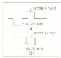
Fig. 3. Oscilloscope display (a) when pulses are not coincident and (b) when pulses are coincident and of equal amplitude.
