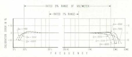
Fig. 2. Effect on voltmeter reading of variation in  $G_m$  in all tubes of Model 400H amplifier. Center  $G_m$  value for tubes used is 6200 micrombos.
