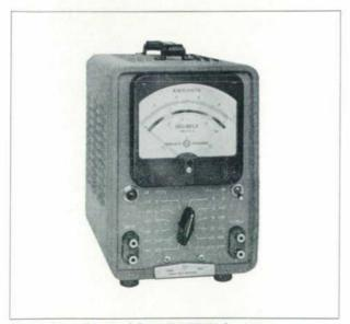
Fig. 1. New -bp- Model 400H VTVM bas 1% accuracy over 50 cps-500 kc range, 2% accuracy over 20 cps-1 mc range, is usable to 4 mc. Mirror scale and bigb-definition meter contribute to accuracy of reading.
