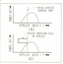
Fig. 4. (a) Typical power output vs. repeller voltage characteristic of klystron used in -bp- microwave generators, (b) Positive modulating pulse applied to repeller circuit pulses klystron out of oscillation.
