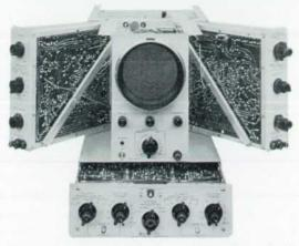
Fig. 13. Model 150A has been designed to afford bigh degree of accessibility to parts as indicated by above view of instrument with cabinet removed.
