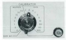
Fig. 12. Calibrator voltage selector and terminal.
