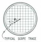
Fig. 7. Representation of typical trace ob-tained when measuring reflection coefficient magnitude with the setup of Fig. 4. Angle formed with the horizontal projection of left point of trace thru origin is proportional to reflection coefficient. Position of left point typically varies with frequency because p varies. Mask or line drawn on tube face with grease pencil can be used to mark a limit for production acceptance tests.
