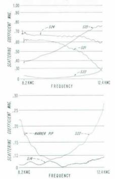
Fig. 6. Records made of magnitude of scattering coefficients of bybrid-tee using arrangements of Figs. 4 and 5. Arms 1 and 4 are H and E arms, respectively, 2 and 3 the side arms. Such records can be made in only a few minutes. Marker pips are from wavemeters and can be used to define frequency ranges of special interest.
