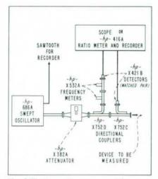
Fig. 4. Equipment arrangement for measuring reflection coefficient magnitude in either permanent form or as viewed on meter or oscillator trace. Wavemeters in incident arms are used to insert marker pips at desired points.
