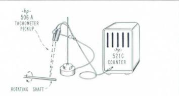
Fig. 2 (above). Counter is arranged to operate with -hp- 506A Tachometer Pickup to measure very high rotary speeds of up to 300,000 rpm without mechanically loading rotating system.
