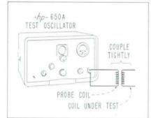
Fig. 5. Self-resonant frequency of small coils can usually be found by coupling coil to Model 650A through a probe coil and sweeping frequency dial for meter dip.
