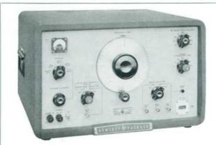
Fig. 1. Besides providing c-w, a-m, and f-m outputs, -hp- Model 686A voltage-tuned oscillator sweeps over full 8.2 – 12.4 kmc range or increments as small as 4.4 mc. Wide range of sweep rates enables measurements to be plotted on recorder or displayed without flicker on oscilloscope. Manual trigger facilitates permanent recording.
