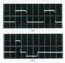
Fig. 7. (a) Oscillogram showing typical quality of output pulses from Model 219B Dual Pulse Unit (1 µsec/cm sweep). Pulses can each be obtained from separate outputs or from common output as shown. Polarity, width, amplitude and spacing of pulses from 219B output unit are individually adjustable as indicated by (b).
