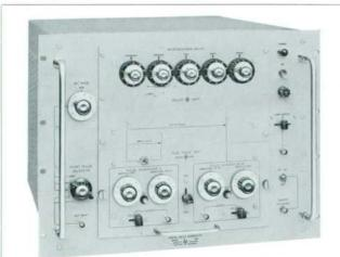
Fig. 1. New hp-Model 218A Digital Delay Generator produces output pulses after digitally adjustable precision intervals of up to 10,000 microseconds on command of external signal to simplify calibrating and testing systems where time interval or delay time is important. Instrument can also count and produce outputs after any de-
