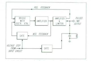
Fig. 4. Block diagram of pulsed crystal oscillator. Ringer is pulsed coincident with oscillator to insure accurate counting of first few cycles of oscillation where small starting transients may exist.
