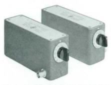
Fig. 1. As a pair, new hp-Models 355A/B 50-ohm Attenuators provide from 0 to 132 db of attenuation in 1 db steps over dc to 500 mc frequency range.
