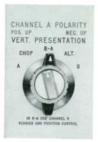
Fig. 3. Vertical presentation selector provides for five types of vertical display. Concentric switch inverts A channel signal to facilitate two-signal comparison.
