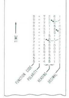
Fig. 4. Typical print-out obtained when voltmeter is used with -hp- digital recorder and operated with a programmer for multi-point measurements. First column identifies measured test point, while remaining columns indicate measured voltage.
