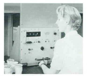
The illustration above shows a typical production operation wherein the new digital voltmeter discussed in the accompanying article facilitates production and reduces operational cost. Here a non-technical operator classifies semiconductor diodes by zener value. Measurements such as this where ordinarily
