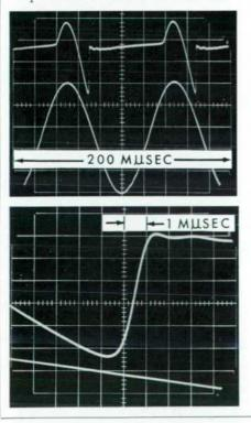
bias as the mechanism of harmonic generation, A. F. Boff of the -hp- laboratories discovered that allowing certain diodes to conduct during a certain portion of the cycle increased the diode conversion efficiency at high harmonics by more than tenfold. Theories brought to bear did not explain the effect or why various diodes differed. Use of conventional oscilloscopes to observe the effect did not provide an answer.
