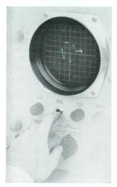
Fig. 3. New "beam-finder" feature enables off-screen trace to be located immediately by pushing panel switch, thus overcoming long-time oscilloscope inconvenience. When switch is depressed, display indicates direction and amount beam is off-center, greatly simplifying adjustment of centering controls.
