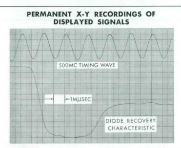
As described in the accompanying article, horizontal deflection in the new oscilloscope is accomplished by a staircase waveform whose steps are synchronized with the pulses that sample the signal being observed. In addition to this automatic scanning, however, provision is also made for scanning to be manually controlled by the operator. Under this arrangement, scanning occurs in proportion to the rotation of a panel control (Scanning - Manual). Combined with this manual scanning provision,
