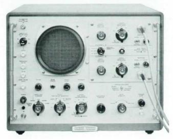
enough so that the overall plot appears continuous. Normally, 1,000 points are plotted per sweep (100 points per centimeter).
