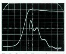
Fig. 9. New Oscilloscope has unusual property of not overloading, as indicated by lower trace in this oscillogram which is same as upper trace except at 20 times as much sensitivity. See text for details.
