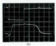
Fig. 10. Oscillograms showing fast switching pulse (upper traces) with resulting mesa transistor output waveform for two degrees of saturation. Time scale is 5 millimicroseconds/cm.
