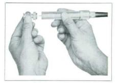
Fig. 16. Adapter being installed to enable signal probe to be connected to BNC type fittings.
