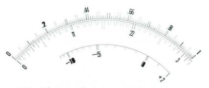
Fig. 4. Scales for two different meters printed by calibrator on one face. Calibrator sets zero and full scale points to same angular position, Difference in tracking error between these end points is clearly evident. Scale reproduced at 90% of full size.
