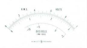
Fig. 2. (above). Typical high accuracy meter scale prepared by calibrator. Scale reproduced at half full size.
