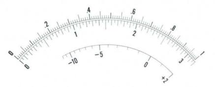
Fig. 3. Reproduction of meter scale processed 5 times by calibrator. Both meter and scale were removed and re-inserted between successive runs. Excellent repeatability of both meter and calibrator are evident here. Scale reproduced at 90% of full size.
