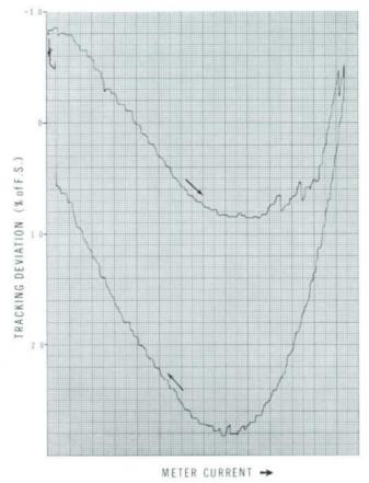
Fig. 7. Tracking deviation characteristic for a meter baving excessive pivot friction.
