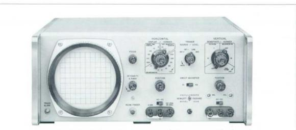
Fig. 1. Internal-graticule cathode-ray tube as used in the new -hp- DC - 450 kc oscilloscope (see p. 3). Locating the graticule on inside of front of tube removes parallax error previously existing with crt's using separate
