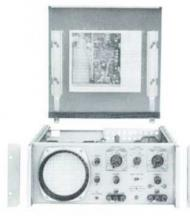
New -hp- Model 120B oscilloscope operates from dc to 450 kc with a vertical system sensitivity of 10 mv/cm. Dual-purpose cabinet can be used either in bench service or can be rack mounted using brackets supplied. Inside of instrument top cover contains large illustration locating most components and all adjustments.
