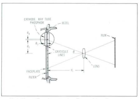
Fig. 2. Diagram illustrating source of parallax error d<sub>4</sub> in oscilloscopes. Since phosphor and graticule in new crt are located in same plane, parallax error is eliminated.
