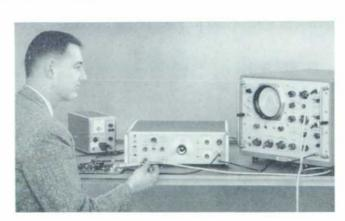
Fig. 1. New hp- Model 215A Pulse Generator (in center) provides pulses as short as 1 nanosecond for general-purpose testing. Pulses are provided at high level and from direct-coupled 50-ohm source for simplicity of external use.
