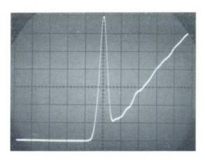
Fig. 1(a) (at left). Oscillogram showing measurement of small inductance of 4" leads on 1000-pf capacitor. Vertical scale is calibrated at 1 nanohenry/cm; sweep speed is 2 nsec/cm.
