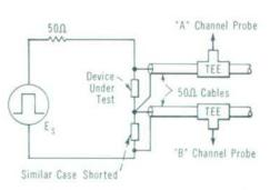
Fig. 7. Arrangement used to separate inberent device overshoot from lead and case inductive responses. Tees are -hp-187B-76E's.
