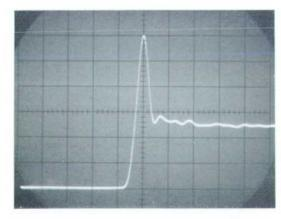
Fig. 6(a). Oscillogram showing spike in measurement of diode lead inductance.
