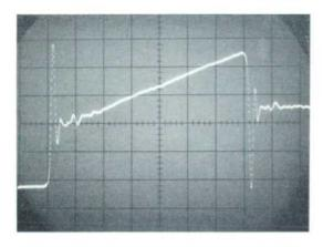
Fig. 8(a) (at left). Oscillograms showing waveforms in measuring small C shunting 1K and 2.2 µb R-L combination. Sweep speed is 5 nsec/cm.
