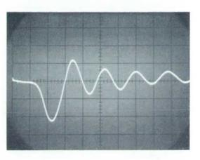
tance gives  $L = (50)^2 (2.5 \times 10^{-12}) =$ 6.25 nanohenries/inch. One inch of this cable, with the far end shorted, was used to obtain the calibrating waveform shown in Fig. 2.
