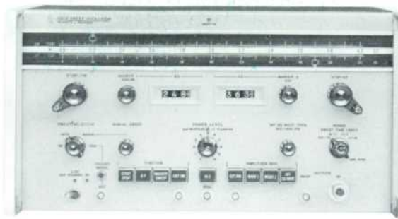
Fig. 3(a). New -hp- Model 692B Sweep Oscillator operates from 2 to 4 Gc. "B" suffix on model number indicates instrument has p-i-n diode type modulator/attenuator in its output circuit for maximum flexibility in modulation and leveling.
