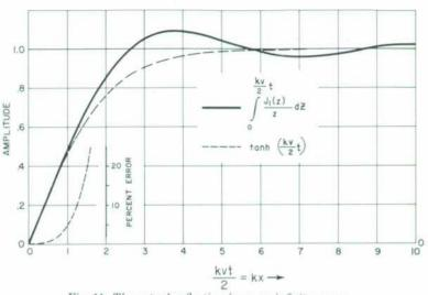
Fig. 11. The actual reflection from an infinite exponentially tapered line (solid), and the line impedance profile plotted on the vertical scale  $y = (Z - Z_0)/(Z + Z_0)$  (dashed curve). The error incurred from reading impedance off the solid curve is under 7% for  $Z/Z_0 < 3$ .
