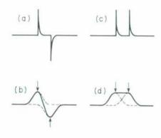
response of this equivalent filter is therefore the derivative of the observed step response.
