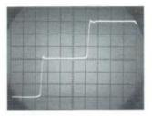
Fig. 13. Three feet of RG-9/Uopen circuited. Sweep speed 2.5 ns/division. The round trip delay is 3.8 divisions or 9.5 nanoseconds. The propagation velocity is thus 193 meters/microsecond or 64% of the velocity of light. The dielectric constant is therefore  $(1/.64)^{\pm}$  or 2.4.
