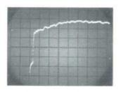
Fig. 18. A long section of lossy 60-ohm line. The jump from 50 ohms to 60 ohms is evident at the start, followed by an irregular rise due to loss and cable dejects. On the vertical scale shown, the incident step would be 35 cm high. Much more vertical magnification could be used without distortion.
