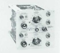
Fast-rise feed-through sampling channels of -hp- 188A dual-channel plug-in for-hp-185A/B Sampling Oscilloscopes bridge 50ohm lines without attenuation.
