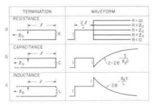
linear the impulse response will be the derivative of the step response, so both waves contain essentially the same information. However, the step response is generally simpler in appearance, easier to interpret, and displays more clearly such things as gradual impedance variation with distance. Unless otherwise noted we will assume a step function test signal.
