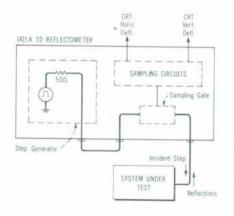
Voltage step generator in -hp- 1415A Plugin connects directly to feed-through sampling channel. Plug-in also has rate generator and necessary synchronizing functions.
