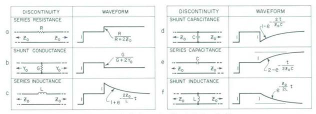
Fig. 6. Typical reflections produced by simple discontinuities.
