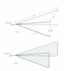
Fig. 20. (a) A V-antenna with two conductors per side tapered to give a constant 300ohm impedance for the first two feet after which the impedance rises. (b) The same antenna with end conductors and mesh added to make side surfaces rather than rods. The sides form a conical 300-ohm transmission line.
