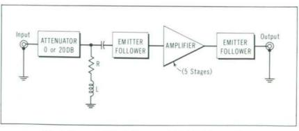
Fig. 5. Elemental block diagram of 461A/462A amplifiers.
