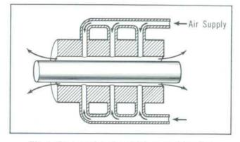
Fig. 4. Cross-section of multiple-venturi bearing.
