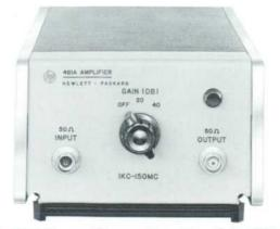
Fig. 3. Model 461A amplifier provides either 40 db (100 ×) or 20 db (10 ×) of broadband gain. Input and output impedances are both 50 ohms.
