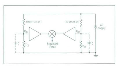
Fig. 8. Electrical analog of one pair of "pads" in multiple-pad bearing of Fig. 7. Capacitances C are added when air or other compressible fluid is used as lubricant. Voltages e<sub>p1</sub> and e<sub>p2</sub> represent pressure within pad.
