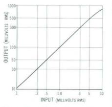
Fig. 4. Transfer characteristics show linearity typical of -hp- Model 461A amplifier.
