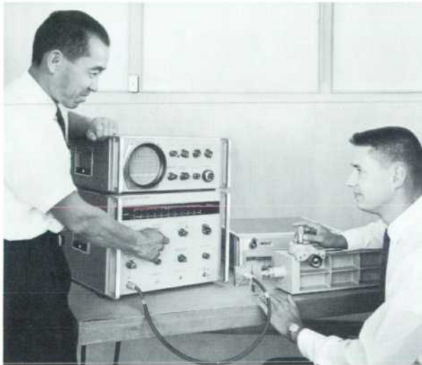
Fig. 1. Hewlett-Packard Model 8551A/851A Microwave Spectrum Analyzer enables evaluation of signals widely separated both in amplitude and frequency. Analyzer here displays harmonic and spurious outputs of frequency doubler throughout range from 10 Mc to above 10 Gc. Doubler generates 3800 Mc output in response to 1900 Mc input and Analyzer clearly shows how mistuning can cause certain diodes to produce non-harmonically related parametric oscillations.
