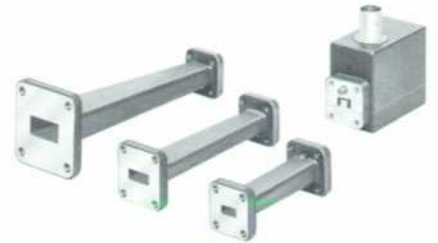
Fig. 8. External mixer connects Spectrum Analyzer to waveguide systems. Two mixers are available, one for X band and one for P, Q and R bands. Taper sections match various waveguide sizes to ridged waveguide of mixer.
