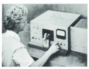
Fig. 1. Special -hp- designed meter-calibrating machine automatically calibrates indicating meters to 1/4% accuracy. Meter being calibrated faces inward on front of machine.
