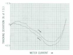
Fig. 2. Typical meter-performance curve (tracking deviation characteristic) measured by -hp- meter calibrator (Fig. 1). Slightness of loop opening shows freedom of calibrated meter from pivot friction; lack of large anomalies in curve shows freedom from stickiness.
