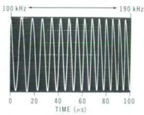
Fig. 7. Oscillogram shows example of swept frequency output of modified synthesizer.
