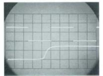
Fig. 4. Reference-phase square-wave output of Function Generator as viewed on oscilloscope triggered by variable-phase square-wave output. Use of variable-phase output as trigger allows reference phase signal to be positioned on CRT as desired. (Upper trace: 20 \(\mu s/cm\).)
