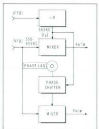
Fig. 15. Variable phase channel has phase shifter in fixed frequency path but otherwise is identical to reference phase channel.
