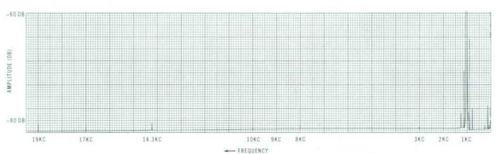
Fig. 6. Typical harmonic content in sine-wave output of Model 203A Function Generator at 1 kc/s shows low distortion in output wave.
