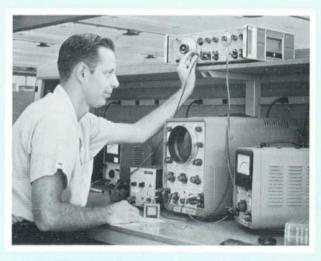
Fig. 1.—hp— Model 203A Variable Phase Function Generator simplifies measurement of gain-phase characteristics of circuits and devices, such as audio driver transformer shown here being checked throughout complete audio range with set-up diagrammed in Fig. 3 and explained in text. New generator has wide frequency range and variable phase outputs adjustable over full 360° range at any output frequency.
