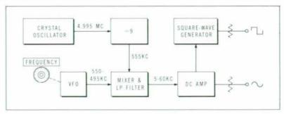
Fig. 10. Simplified block diagram of reference phase channel in -hp- Model 203A Function Generator while operating on highest frequency range (5-60 kc/s).
