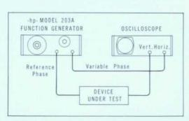
Fig. 3. Set-up for phase-shift measurements using variable phase output achieves sharply defined null (see Fig. 9).
