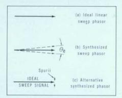
Fig. 10. Representation of frequency sweep by phasors. Phasor representing synthesized sweep (b) oscillates back and forth through peak-to-peak phase error θ, and may be represented by vector addition of ideal sweep phasor and small amplitude-modulated signal in phase quadrature (c).
