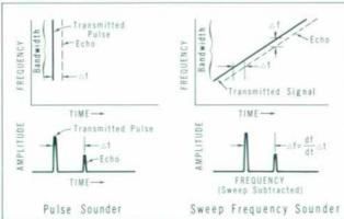
Fig. 3. Frequency-time representation of pulse and Chirp radar signals. Time delay \Delta t of Chirp radar echo is derived from frequency difference \( \Delta \) between transmitted and received signals.
