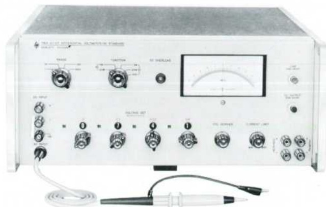
Fig. 4. New -hp- Model 741A AC/DC Differential Voltmeter/DC Standard has low capacitance probe for ac input. Probe and dc input and output are floating. Four VOLTAGE SET controls set resistive divider and push-buttons concentric with VOLTAGE SET knobs select sensitivity of front panel meter. RANGE switch sets illuminated decimal point indicators. OVERLOAD indicator lights if input voltage exceeds selected range or if output current exceeds selected limit. Overload protection to 1000 volts is provided on all ranges.
