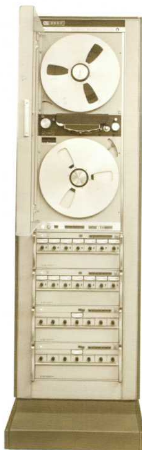
Fig. 1. Low-impedance preamplifiers used in the new -hp- 3950 Series Tape Recorders sense current output of the reproduce heads instead of voltage. The result is a signal-to-noise ratio of greater than 30 dB from 400 Hz to 1.5 MHz, and a greater design flexibility permitting lower system cost, while maintaining high performance. The system is available with up to fourteen record and reproduce channels as shown.
