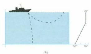
Fig. 1. Bending of a transmitted sonar beam (a) is caused by a combination of a gradual temperature change and a change in density of the water. At certain times of day, and after a storm, mixing occurs at the surface which results in a constant temperature zone. Under this condition, a sonar beam launched at an angle may return to the
