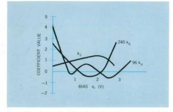
Fig. 5. Second, fourth, and sixth-power coefficients of hypothetical diode characteristic of Fig. 4. Biasing one diode of balanced mixer at 1V and the other at 2V makes  $k_{\epsilon}$ 's cancel and  $k_{\epsilon}$ 's = 0, but changes desired coefficient  $k_{\epsilon}$  by only a few dB.
