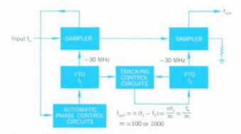
Fig. 2. Simplified block diagram of automatic frequency divider. Control circuits maintain indicated relationships between  $f_{z}$ ,  $f_{1}$ , and  $f_{2}$ .
