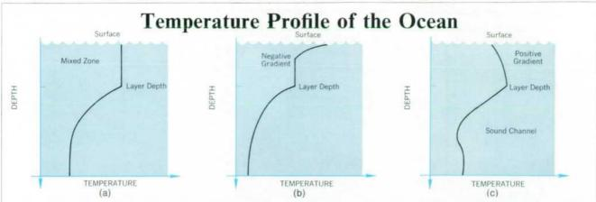
The oceans are characterized by three distinct layers: (a) an upper layer normally isothermal due to mixing by winds, a middle (thermocline) region of strong negative gradients, and a lower region of slow change extending to the bottom; (b) illustrates the 'afternoon effect' when summer heat and light winds can cause a negative gradient in the upper layer. A positive gradient (c) can also form when cool,
