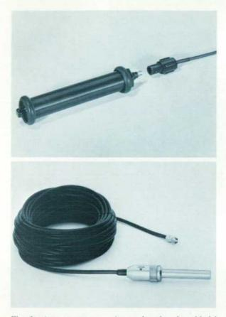
Fig. 3. A temperature sensing probe, the -hp-Model2832A, top, houses the quartz crystal and all electronics in a pressure case designed specifically for measurement of ocean temperatures. At the bottom, the -hp-Model2833A sensor assembly in a stainless steel case will withstand pressures to 10,000 psi and may be operated at distances up to one mile from the temperature readout.
