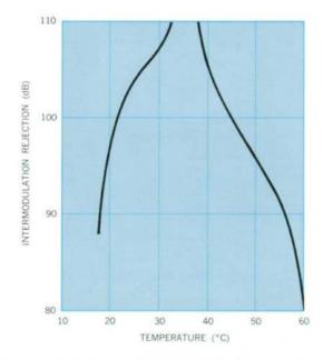
Fig. 6. Temperature dependence of IM rejection of a balanced hot-carrier-diode mixer.
