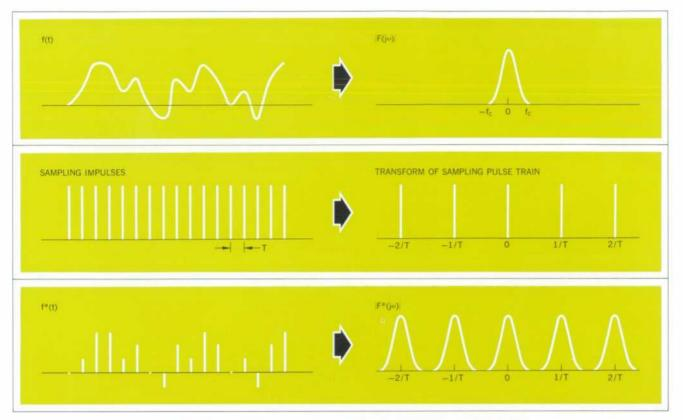
Fig. 5. Band-limited signal (top) sampled by infinite impulse train (middle) has frequency spectrum consisting of original spectrum duplicated at multiples of sampling frequency 1/T. No information about signal is lost as long as duplicate spectra do not overlap, i.e., as long as 1/T >2f<sub>c</sub>, where f<sub>c</sub> is highest frequency present in signal f(t).
