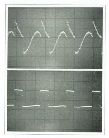
Fig. 4. Top: 200.0-Hz rectangular wave plus 200.1-Hz sine wave, before averaging. Bottom: 200.0-Hz rectangular wave recovered by signal averager after 2<sup>14</sup> repetitions. In this case, averager had the effect of a comb filter whose teeth had 3-dB bandwidths of 0.0027 Hz.
