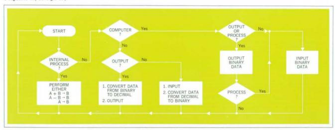
Fig. 2. I/O coupler provides digital display, input and output data transfers, and simple processing of data stored in memory of HP 5480A Signal Analyzer.
