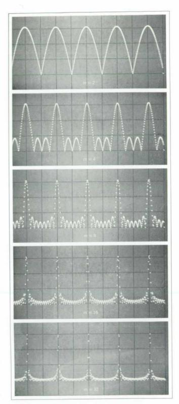
Fig. 3. Effective transfer function of signal averager, calculated by digital computer. Averager acts like comb filter for repetitive waveforms. Since averager is time-locked to repetitive waveform, frequency components of waveform coincide exactly with centers of comb-filter teeth. Width of teeth is inversely proportional to number of repetitions averaged.
