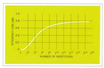
Fig. 3. For same number of repetitions, noise attenuation given by stable averaging is slightly less than that given by summation. Difference, or efficiency loss, grows asymptotically to 0.77 dB.
