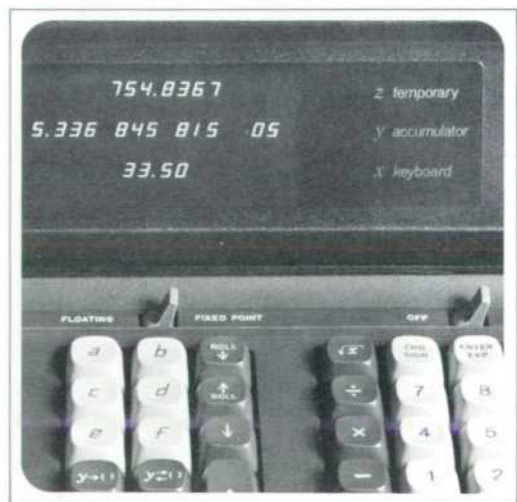
Fig. 1. (left) This new HP Model 9100A Calculator is self-contained and is capable of performing functions previously possible only with larger computers. Fig. 2. (right) Display in fixed point with the decimal wheel set at 5. The Y register has reverted to floating point because the number is too large to be properly displayed unless the digits called for by the DECIMAL DIGITS setting is reduced.
