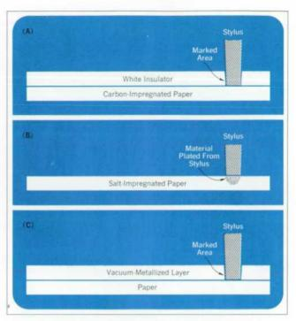
Fig. 4. Carbon-impregnated paper (top) is marked by raising the stylus voltage across the coating to the point of dielectric breakdown, removing the white insulating layer. The salt-impregnated paper (middle) is marked by electroplating stylus material onto the surface of the paper. Vacuum metallized papers (bottom) are marked by fuzing away the metallized layer.
