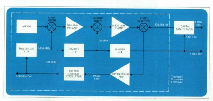
Fig. 4. The hydrogen maser's output frequency is 1420.405 751 786 4 MHz and its output power level is typically -97 dBm. Here is a system for obtaining 100-MHz, 5-MHz, and 1-MHz outputs at useful power levels.
