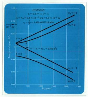
Fig. 3. In the hydrogen maser, the desired transition is from energy state F=1,  $m_{\rm F}=0$  to energy state F=0. The energy of this transition, and therefore the maser's operating frequency  $\nu$ , depend upon the magnetic field  $B_{\rm c}$ , so maser cavities are carefully shielded to eliminate stray fields.
