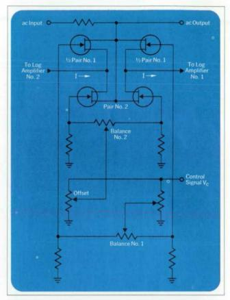
Fig. 7. Using field-effect transistors as variable resistors, the electronic attenuator can vary its resistance over more than an 80 dB range, from about 30  $\Omega$  to 1 M $\Omega$ , in response to a control voltage.
