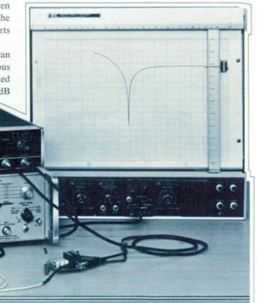
Fig. 1. New model 7562A Logarithmic Converter can be used with Model 3300A/3305A Sweep Oscillator to make frequency response plots over an 80 dB amplitude range and a four-decade frequency range. The converter produces a dc output voltage proportional to the logarithm of the rms value of an ac input signal. Its frequency range is 0.5 Hz to 100 kHz. It can also convert dc signals.
